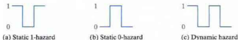
FIGURE 9.34 Types of hazards
