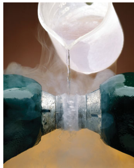
Richard Megna/Fundamental Photographs Liquid oxygen is suspended between the two pole faces of a magnet because the liquid is paramagnetic and is magnetically attracted to the magnet.
