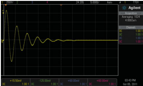
Courtesy Agilent Technologies Figure 31-3 An oscilloscope trace showing how the oscillations in an RLC circuit actually die away because energy is dissipated in the resistor as thermal energy.
