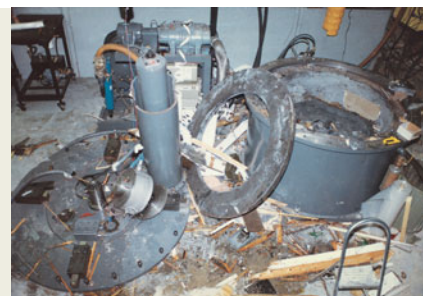
Figure 10-15 Some of the destruction caused by the explosion of a rapidly rotating steel disk.
