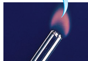
Hydrogen burning in air to form water.
