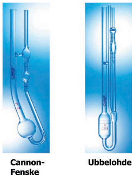
Figure 22. Cannon-Fenske and Ubbelohde capillary viscometers (courtesy of Cannon Instrument Company)
