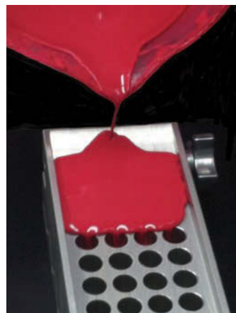
Figure 1. Melted lipstick being poured into metal split mold
