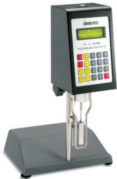
Figure 8. Brookfield DV-III Ultra viscometer (reprinted by permission from Brookfield Engineering)
