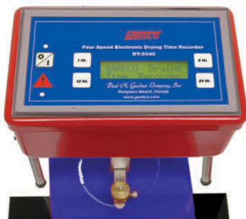
Figure 27a. Digital Drying Time Recorder Photo courtesy of Paul N. Gardner Co.
