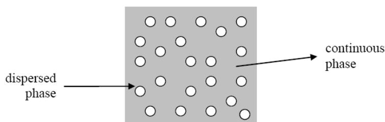
Figure 1: emulsions are a mixture of immiscible substances: an internally suspended dispersed phase, and an external continuous phase
