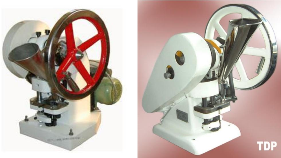
**Gambar 2.** Mesin *single punch*
