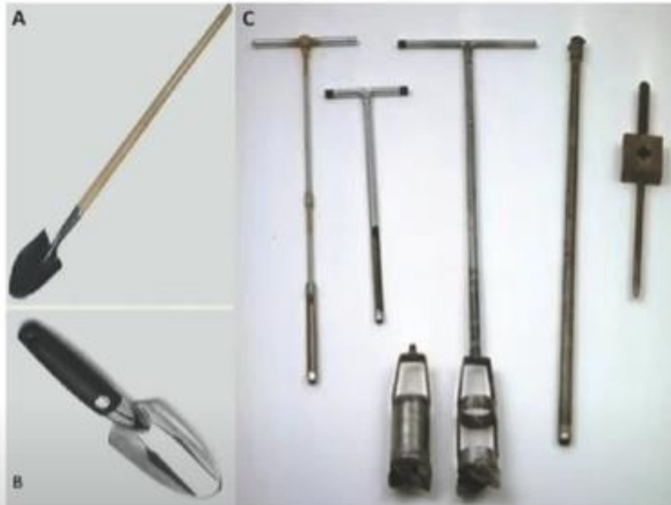
Shovels and other devices used for collecting soil samples. (A) Classic point-shovel. (B) hand shovel. (C) From left to right: Viehmeier tube, trowel, oakfield tubes, soil corers
