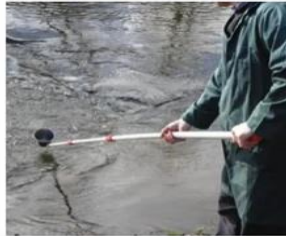
the TeleScoop is our popular extendable device for liquid sampling
