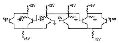
Fig. 4.41. A complementary current switch flip-flop
