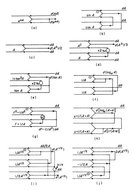
Fig. 8.3. Generation of functions by means of integrators.
