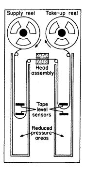
Fig. A.3. Magnetic tape transport with slack tape formed by air pressure
