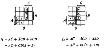
Fig. 3.9. Alternate expressions based on different groupings of a function are formed, resulting in different but equivalent expressions,  $f_1$  and  $f_2$ .
