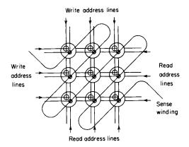
Fig. 5.18. A coincident-current transfluxor storage array
