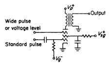
Fig. 4.13. Pentode pulse gate
