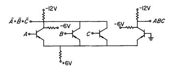
Fig. 4.40. A p-n-p complementary current switch gate
