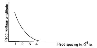
Fig. 5.3. Read voltage variation with head spacing
