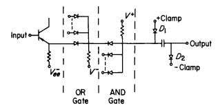
Fig. 4.23. A transistor driven diode gating network
