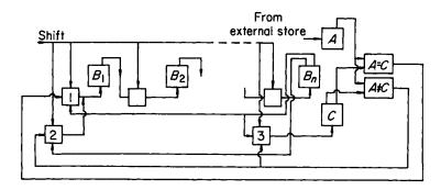
Fig. 6.17. An alternate logical scheme for serial addition utilizing a shift register for augend-sum storage
