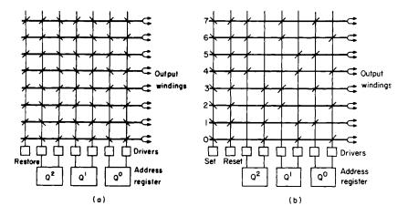
Fig. 5.14. (a) Multicoincidence magnetic core switch, (b) biased multicoincidence magnetic core switch
