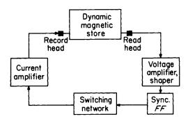
Fig. 5.10. Record-read system for one channel of a dynamic magnetic store
