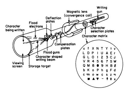
Fig. A.4. Simplified schematic of the Typotron (courtesy of Hughes Aircraft Co.) at the rate of about 20,000 characters/sec. In each, a metal stencil
