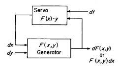
Fig. 8.21. Use of a digital servo for function inversion
