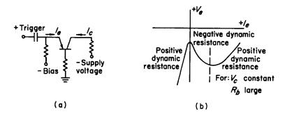
Fig. 4.18. (a) Single point-contact transistor flip-flop, and (b) Voltage-current characteristic of emitter circuit
