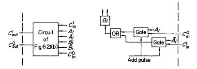
Fig. 6.27. Typical stage of an accumulator with a 0 and 1 carry propagation circuit
