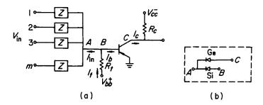
Fig. 4.27. (a) Basic transistor NOR circuit (p-n-p type), and (b) Modification for higher speed operation
