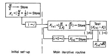
Fig. 2.4. Flow design for a square root program
