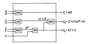
Fig. 3.4. A Combinational switching network
