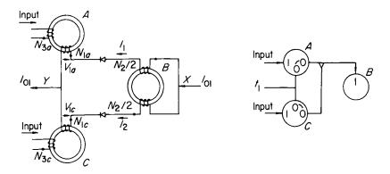
Fig. 4.54. Schematic and symbolic representation of an inhibit transfer loop
