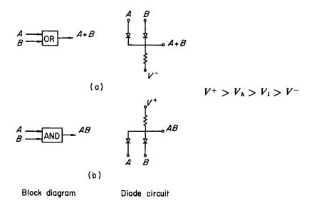
Fig. 4.4. Single level gates
