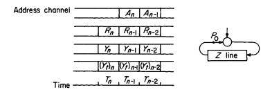
Fig. 8.9. Relative locations of address decoding information and other data in a serial DDA
