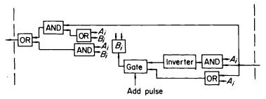
Fig. 6.26. Typical stage of a parallel accumulator with no carry command input
