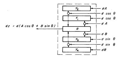
Fig. 8.29. Block diagram of a five-line operational unit.
