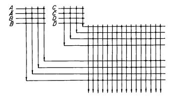
Fig. 4.69. The most economical form of a four-input many-to-one switching matrix
