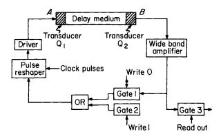
Fig. 5.27. Block diagram of an acoustic delay line store
