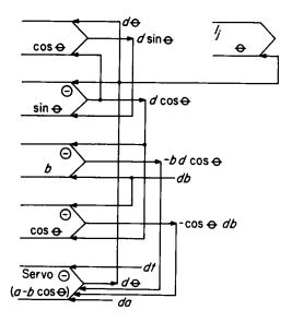
Fig. 8.22. Generation of  $(\cos^{-1})$  utilizing a digital servo
