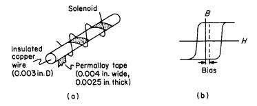
Fig. 5.19. Twistor storage element: (a) physical form and (b) hysteresis loop showing bias due to open magnetic structure
