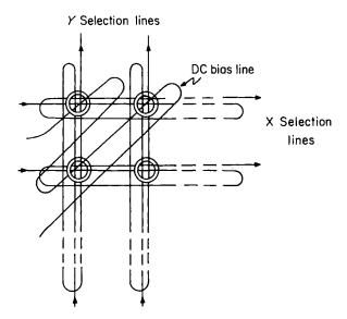
Fig. 5.13. Biased coincident-current magnetic core switch
