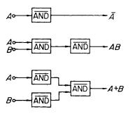
Fig. 3.2. Derivation of primitive logical operations by AND operators only
