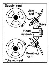
Fig. A.2. Magnetic tape transport with slack tape formed by zig-zag loops and movable arms
