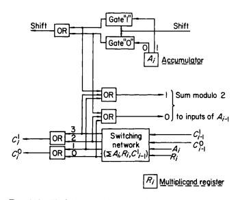
Fig. 6.32. Typical stage of an asynchronous binary multiplier
