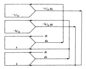
Fig. 8.10. A mapping for solution of the equation:  $a \frac{d^2x}{dt^2} + b \frac{dx}{dt} + cx = 0$
