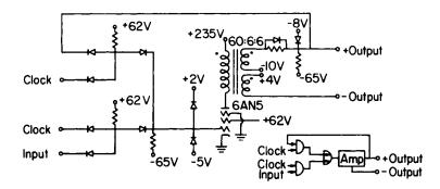
Fig. 4.14. Circuit and block diagram of a pulse gate and regeneration circuit for an ac system
