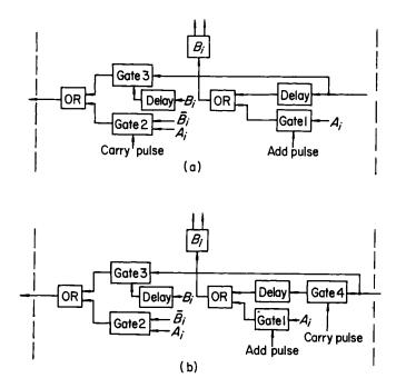
Fig. 6.22. Typical stage of a parallel accumulator. (Either one but not both delay units may be required in these two arrangements.)
