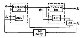
Fig. 6.12. An adder suitable for use with a recirculating type of main store
