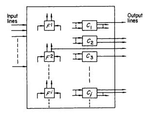
Fig. 3.17. Model of a sequential switching network. (F = storage element, C = combinational circuit)
