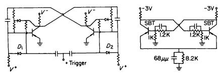
Fig. 4.34. A nonsaturating flip-flop
