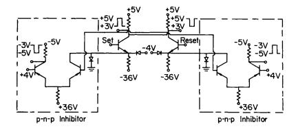
Fig. 4.46. A complementary current flip-flop with four outputs
