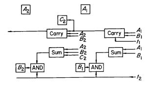
Fig. 6.20. A parallel adder with flip-flop storage and an anticipatory carry chain
