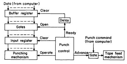
Fig. A.1. Block diagram of paper tape punch timing control
