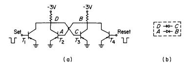
Fig. 4.30. Basic DCTL flip-flop with input circuits
