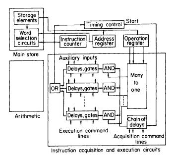
Fig. 7.6. Asynchronous control for a single-address GP computer
