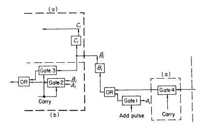
Fig. 6.23. Typical stage of a parallel accumulator
