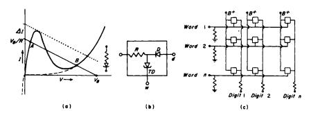
Fig. 5.22. (a) Tunnel-diode characteristic curve, (b) three-element memory cell, (c) linear array of three-element cells.
