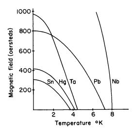
Fig. 4.62. Critical magnetic field,  $H_c$ , curves for several superconductors
