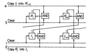
Fig. 4.75. A high speed dc coupled shift register with flip-flop intermediate storage
