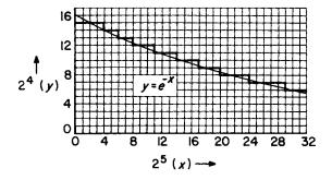
Fig. 8.7. Generation of  $e^{-x}$  by a digital integrator
