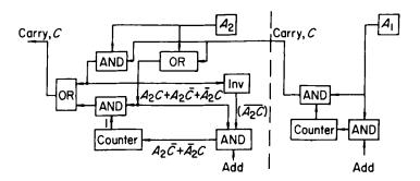
Fig. 6.19. A parallel adder with bistable counter storage and an anticipatory carry chain
