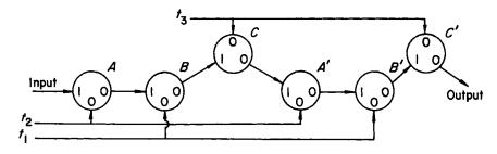
Fig. 4.79. A serial shift register using three cores per two bits and single diode transfer loops
