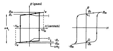
Fig. 4.47. Idealized hysteresis loop of a ferromagnetic material
