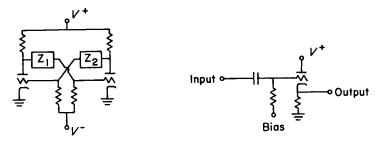
Fig. 4.11. Basic vacuum tube static flip-flop circuit
