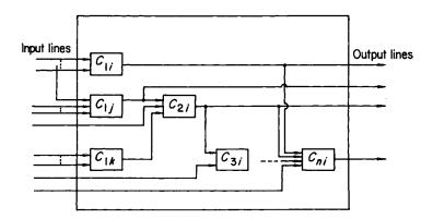
Fig. 3.3. Model of a combinational switching network
