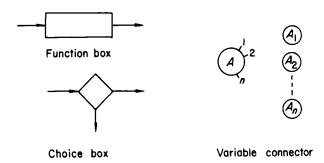
Fig. 2.5. A basic set of symbols for a flow diagram
