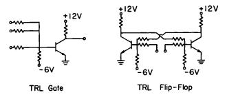
Fig. 4.28. Basic transistor-resistor logic circuits (n-p-n type)
