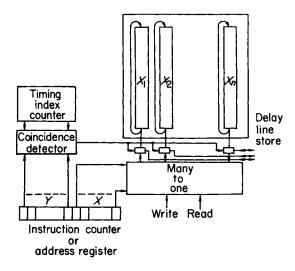
Fig. 7.3. Word selection in a delay line store
