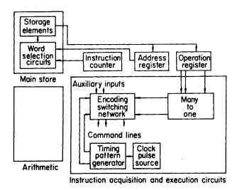
Fig. 7.5. Synchronous control for a single-address GP computer
