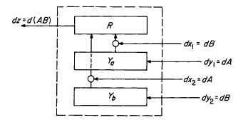
Fig. 8.26. Block diagram of a three-line structure programmed as a multiplier.
