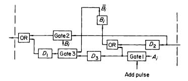
Fig. 6.25. Typical stage of a parallel accumulator with no carry command input
