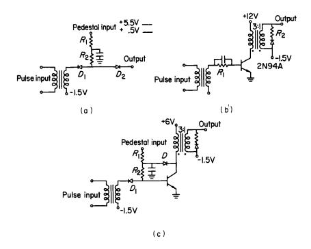
Fig. 4.38. A gated pulse amplifier system of circuit logic, (a) pulse-pedestal gate, (b) pulse amplifier, (c) combined pulse-pedestal gate and pulse amplifier.
