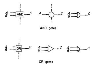
Fig. 4.1. Functional representations of AND and OR gates
