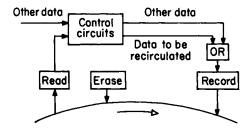
Fig. 5.5. A head arrangement for two-level RZ recording
