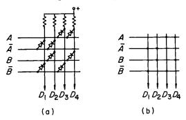
Fig. 4.65. Representations of a many-to-one rectangular switching matrix with two input variables
