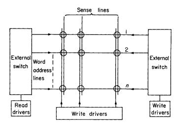
Fig. 5.16. Linear selection: word organized magnetic core storage array
