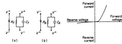
Fig. 4.2. Equivalent circuits of a semiconductor diode
