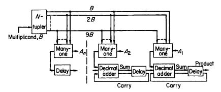
Fig. 6.34. A serial-parallel decimal multiplier
