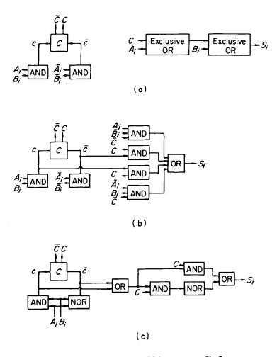
Fig. 6.14. Three adders utilizing a carry flip-flop
