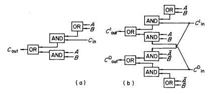
Fig. 6.21. (a) A simple carry circuit, (b) A circuit to propagate 0 and 1 carries
