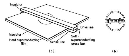
Fig. 5.21. Persistent-supercurrent thin film storage cell: (a) physical form, (b) path of circulating currents
