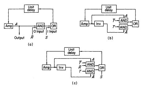
Fig. 3.16. Dynamic flip-flops: (a) set-reset type, (b) trigger type, (c) set-reset-complement type. [Amp denotes an amplifier. Inv denotes an inverter which amplifies and complements a signal. The unit delay is provided by an electromagnetic delay line].
