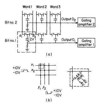
Fig. 5.31. Diode capacitor storage array, (a), and transformer AND gate selection matrix, (b)
