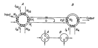
Fig. 4.52. Schematic and symbolic representation of a single diode transfer loop
