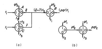
Fig. 4.57. (a) Magnetic core AND gate formed from "negation" circuits, and (b) magnetic core AND gate
