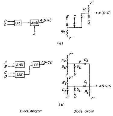
Fig. 4.5. Two-level gates
