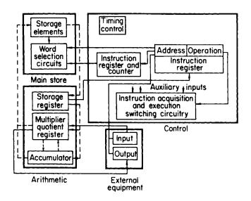
Fig. 7.4. Over-all arrangement for a single-address GP computer
