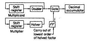
Fig. 6.35. Decimal multiplication by halving one factor, doubling the other
