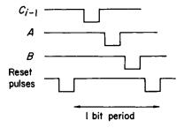
Fig. 6.8. Relative timing of signals to a sum and carry producing counter
