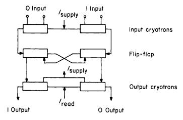
Fig. 4.64. Cryotron flip-flop with input and output cryotrons
