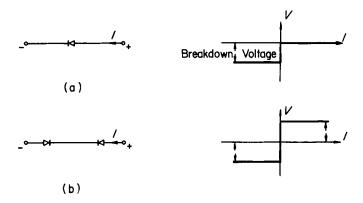
Fig. 4.31. Volt-ampere characteristics of idealized breakdown diodes
