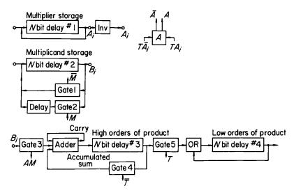
Fig. 6.29. A serial binary multiplier with delay line storage
