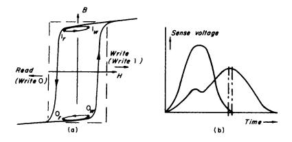
Fig. 5.12 (a) Minor hysteresis loops from half-select signals, (b) strobing of sense voltage.
