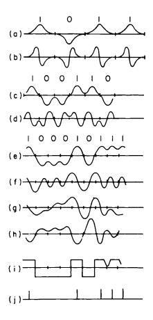
Fig. 5.6. Read waveforms in RZ recording for various recording densities,  $p_i$
