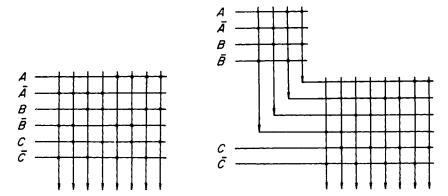
Fig. 4.66. A many-to-one rectangular switching matrix with three input variables
