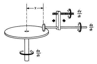
Fig. 8.2. Schematic of a mechanical integrator
