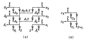
Fig. 6.1. Diode gating network for generating input signals to a three stage binary counter composed of (a) R-S flip-flops, (b) T flip-flops
