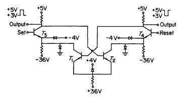
Fig. 4.45. Simplified complementary current flip-flop
