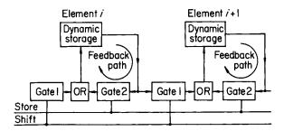
Fig. 4.77. Shift register comprised of dynamic storage elements
