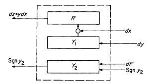
Fig. 8.27. Block diagram of a three-line structure programmed as an integrator and servo register.
