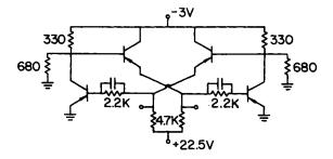
Fig. 4.36. A saturating emitter follower coupled flip-flop
