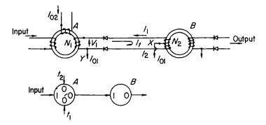
Fig. 4.53. Schematic and symbolic representation of a split winding transfer loop
