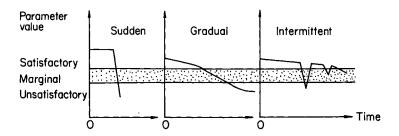
Fig. 9.2. Different types of failure
