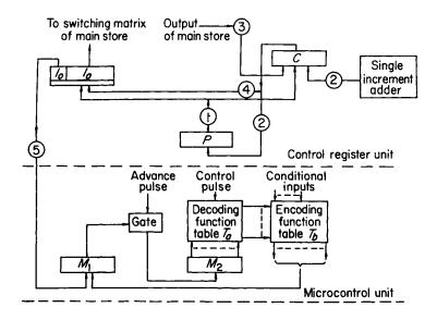
Fig. 7.7. A microprogrammed control unit
