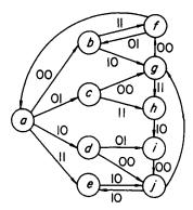
Fig. 3.18. Superstates and permissible superstate sequences of a sequential switching network
