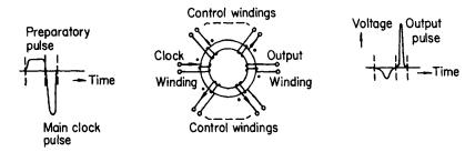
Fig. 4.58. A multi-input magnetic core gate showing the clock and output waveforms
