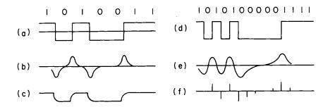
Fig. 5.7. Record and read waveforms in NRZ recording
