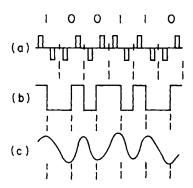
Fig. 5.8. Record and read waveforms in Ferranti phase modulation recording
