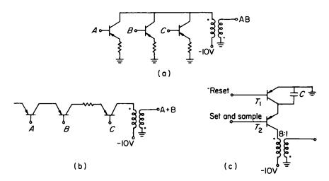
Fig. 4.37. A dynamic pulse system of circuit logic
