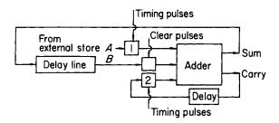
Fig. 6.15. A serial adder utilizing a delay line for augend-sum storage
