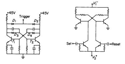
Fig. 4.32. A nonsaturating binary counter
