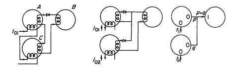
Fig. 4.55. Magnetic core or gate with single advance pulse input
