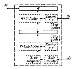
Fig. 8.4. Block diagram of a digital integrator
