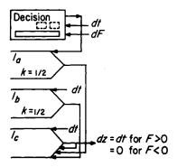
Fig. 8.16. Decision unit (type 2) controlled by a variable F
