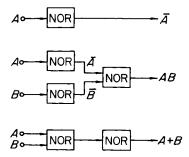
Fig. 3.1. Derivation of primitive logical operations by NOR operators only
