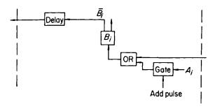
Fig. 6.24. Typical stage of a parallel accumulator with no carry command input
