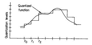
Fig. 1.1. Quantization of a function
