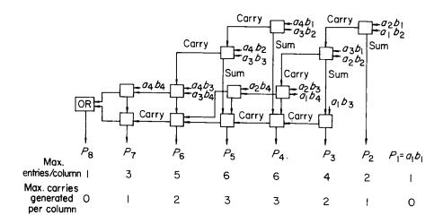
Fig. 6.33. A simultaneous binary multiplier
