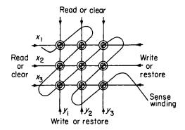
Fig. 5.11. Coincident current magnetic core storage array, showing directions of current flow for read or clear, and write or restore operations
