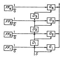
Fig. 4.72. Schematic of a collection unit
