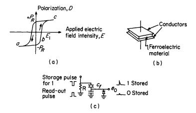
Fig. 5.32. Ferroelectric storage, (a) polarization hysteresis curve, (b) storage cell, (c) read-out circuit
