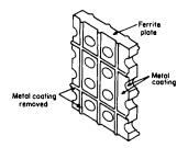
Fig. 5.17. Section of apertured ferrite plate
