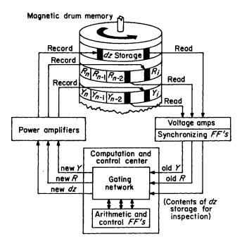
Fig. 8.8. Information flow through a completely serial digital differential analyzer (external inputs and outputs not shown)
