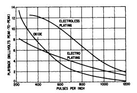
Fig. 5.9. Read voltage variation with recording density for three types of magnetic coatings (Courtesy of Remington-Rand UNIVAC; Jacoby, M. [1962])
