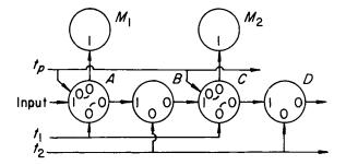
Fig. 4.80. A parallel shift register with single diode and split winding transfer loops
