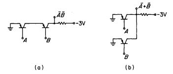
Fig. 4.29. Surface barrier transistor logic circuits: (a) NOR, (b) Sheffer stroke
