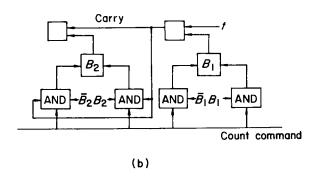
Fig. 6.3. Multistage counters with a two-input/stage carry propagation line, (a) using bistable counter circuits, (b) using R-S flip-flops
