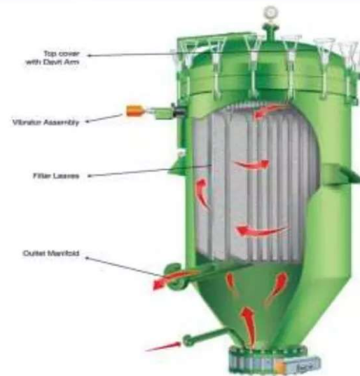
Vertical Pressure Leaf Filter
