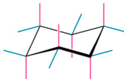
FIGURE 4.11 A procedure for drawing axial and equatorial bonds in chair cyclohexane.
