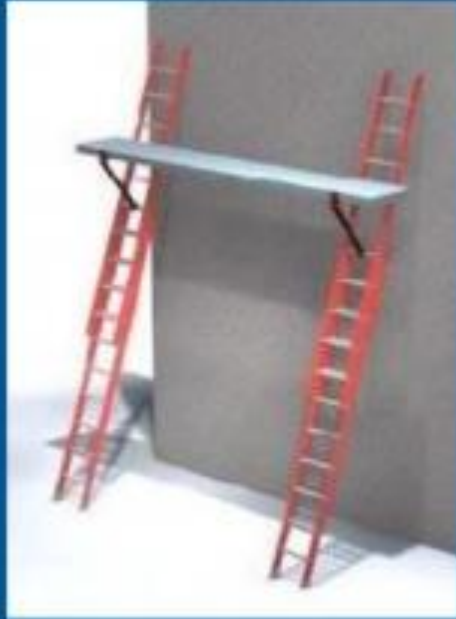
Ladder jack scaffold
