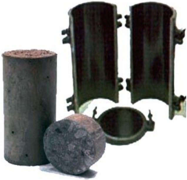
SAMPLE SILINDER H = 30 CM DIAMETER = 15 CM
