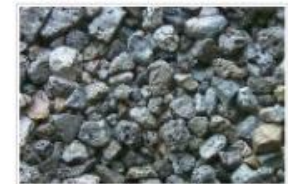
An open graded coarse aggregate, produced by crushing and screening air-cooled iron Blast Furnace Slag
